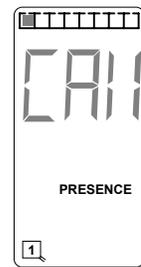
**Step 1:** Observe a single standard automobile in the loop zone. Note the number of segments displayed on the bargraph. **(4)**
